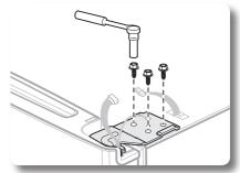
3. With the 10mm wrench, remove the three bolts that hold the hinge on the top of the refrigerator.
